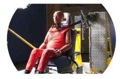
**Crash Simulation sleds** for passive safety components development or Conformity of Production (COP) tests. Different propulsion and deceleration technologies are available to match with each customer needs.
