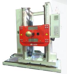
**Multi Launcher** Flexible positioning frames for many different type of test, either free flight or guided (head forms, leg forms, upperleg forms, boby block, pendulum, ejection mitigation, misuse, knee impact...
